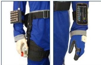
Figure 4: Wearable distributed user interfaces enable users to operate their mobile systems in settings where touch operation is unsuitable. They are also used to operate wearable systems such as VR systems.
