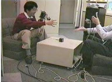
Figure 1. "Transvision" [7], a design tool where collaborators look on a real table-top through a palmtop size see-through display. 3D data from the display is process by an external graphics workstation.
