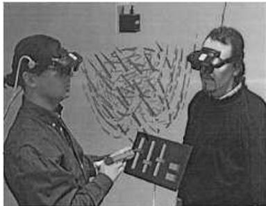
Figure 2. "Studierstube" [8], a system capable to visualize three-dimensional scientific data with see-through glasses. Tracking data is processed on an extra tracking server.
